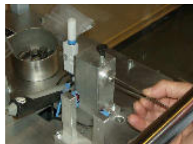
Placing of the cold sample on his pumping support where the robot will pick it up.
