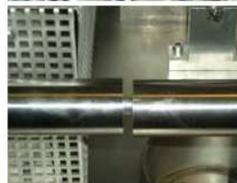
The sample has been finally placed between the Hopkinson bars
