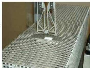
Placing of the cold sample on his pumping support where the robot will pick it up.
