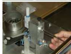
Placing of the cold sample on his pumping support where the robot will pick it up.
